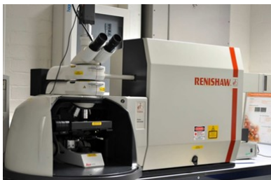
A Raman microscope that is used for the analysis of our samples
